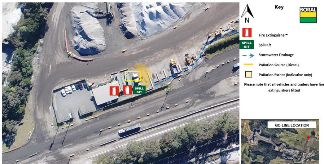
Figure 4: DSS Go-line Area Incident 1: Diesel/Hydrocarbon Spill
