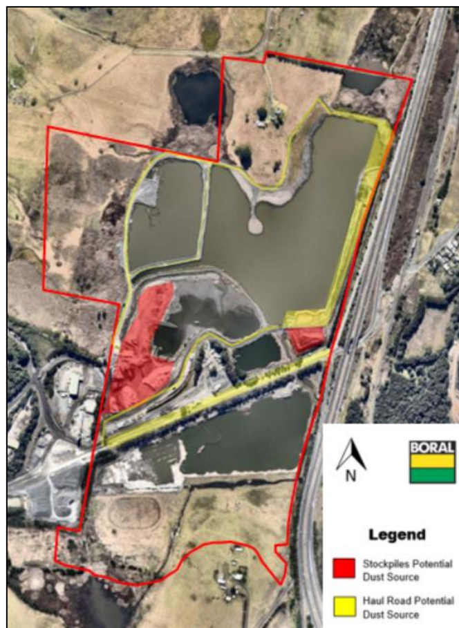
Figure 6: Incident 2: Sources of Dust Pollution at Dunmore Sand and Soil
